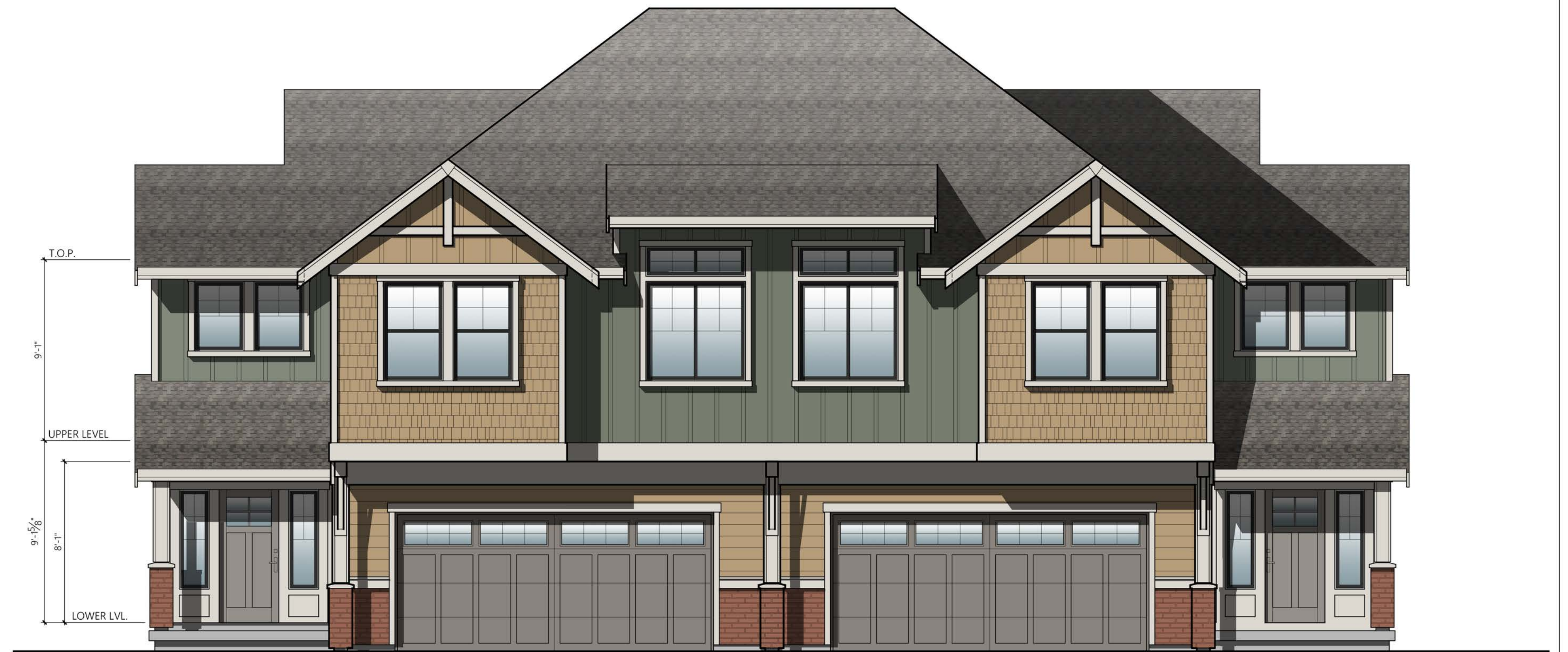
TYPICAL 2 STORY ELEVATION FRONT ELEVATION 1/4" = 1'-0"
