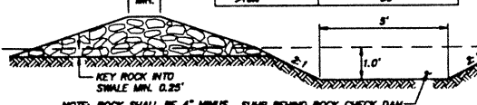
ROCK CHECK DAM CROSS SECTION ROCK CHECK DAM DETAILS NOT TO SCALE
