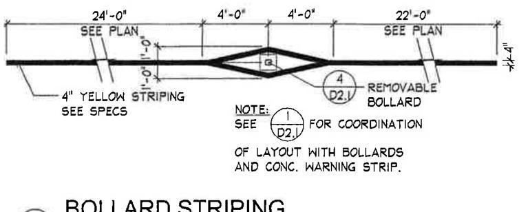
**BOLLARD STRIPING** 5 SCALE: 1/4" = 1'-0"
